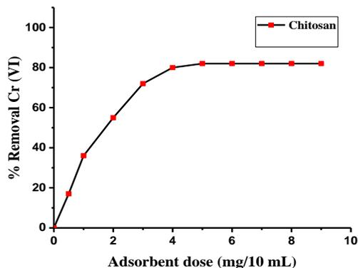
**Figure 7.** Removal percentage of hexavalent chromium by chitosan. Experimental conditions: at different dose, initial concentration 5 mg/L, PH 1 and temperature  $25 \pm 2$  °C.
