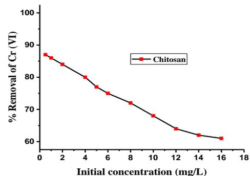
**Figure 5.** Effect of initial concentration on the removal percentage of hexavalent chromium by chitosan.
