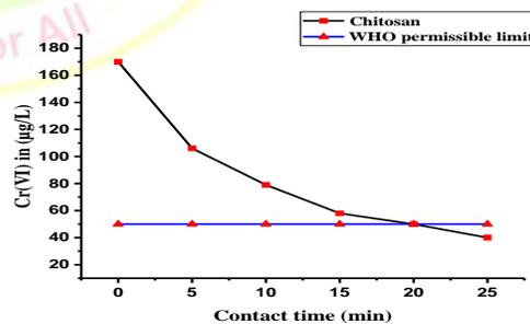
**Figure 9.** Concentration-time profile for the removal of 170 µg/L of Cr(VI) ions from the collected tannery wastewater sample by using chitosan adsorbent.
