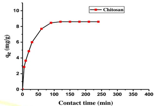
**Figure 4.** Adsorption capacity of hexavalent chromium by chitosan. Experimental conditions: adsorbent dose 5 mg/ 10 mL, PH 1 and temperature  $25 \pm 2^\circ\text{C}$ .
