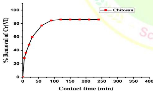
**Figure 3.** Removal percentage of hexavalent chromium by chitosan. Experimental conditions: adsorbent dose 5 mg/ 10 mL, PH 1 and temperature  $25 \pm 2^\circ\text{C}$ .
