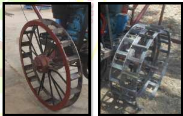
Fig. 12. View of Traction cage wheel (A) existing (B) modified
