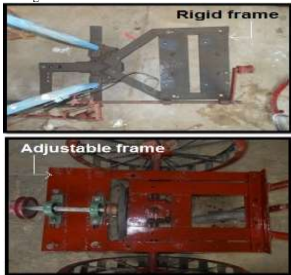
Fig 9. Alignment of frame in (A) existing model (B) modified model
